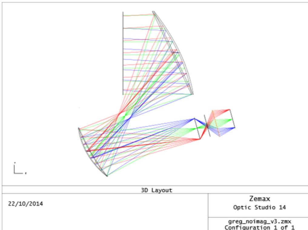
Figure 3: Gregorian design with re-imaging optics
