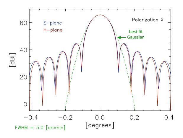
feed = perfect Gaussian beam with no cross-polarization taper = -3 dB, taper angle = 15 degrees
