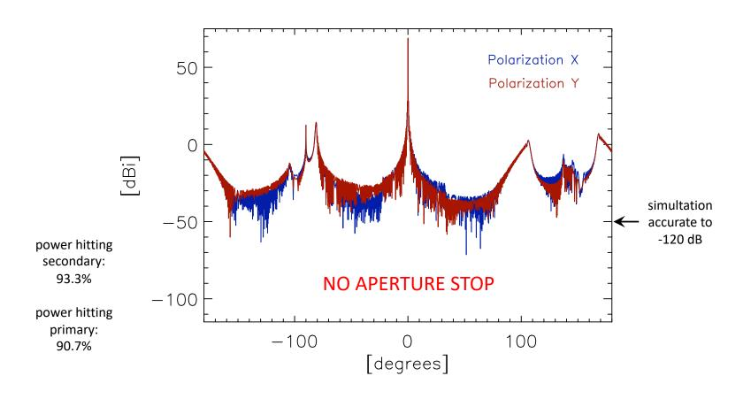
pattern from feed and currents on primary and secondary mirrors
