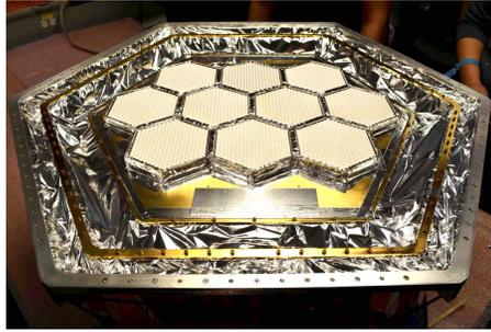
Figure 5.1: SPT-3G operates a focal plane with sinuous antenna-coupled, three-band pixels with 16,000 bolometers [103]. Each pixel couples radiation to bands at 95, 150, and 220 GHz.
