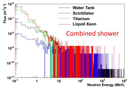
Neutrons cross the the outer boundary (out-->in) of the water tank, scintillator, titanium and liquid Xe volume.
