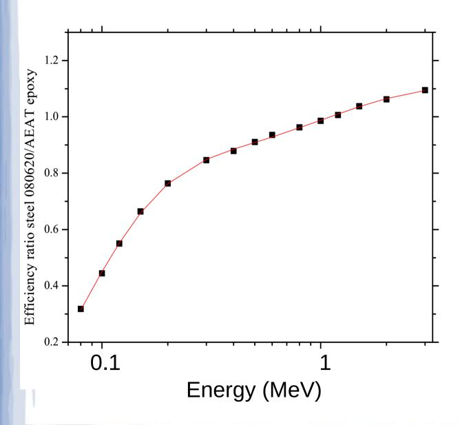
Efficiency correction for steel sample.
