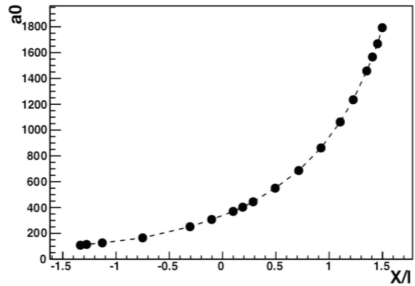
Calibration with Na22(1.27MeV). Place the source on the tube and change it each 2.5 cm.
