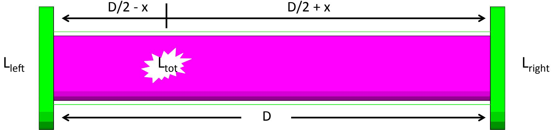
$$L_{\text{left}} = 0.5L_{\text{tot}}e^{-(D/2-x)/l}$$
