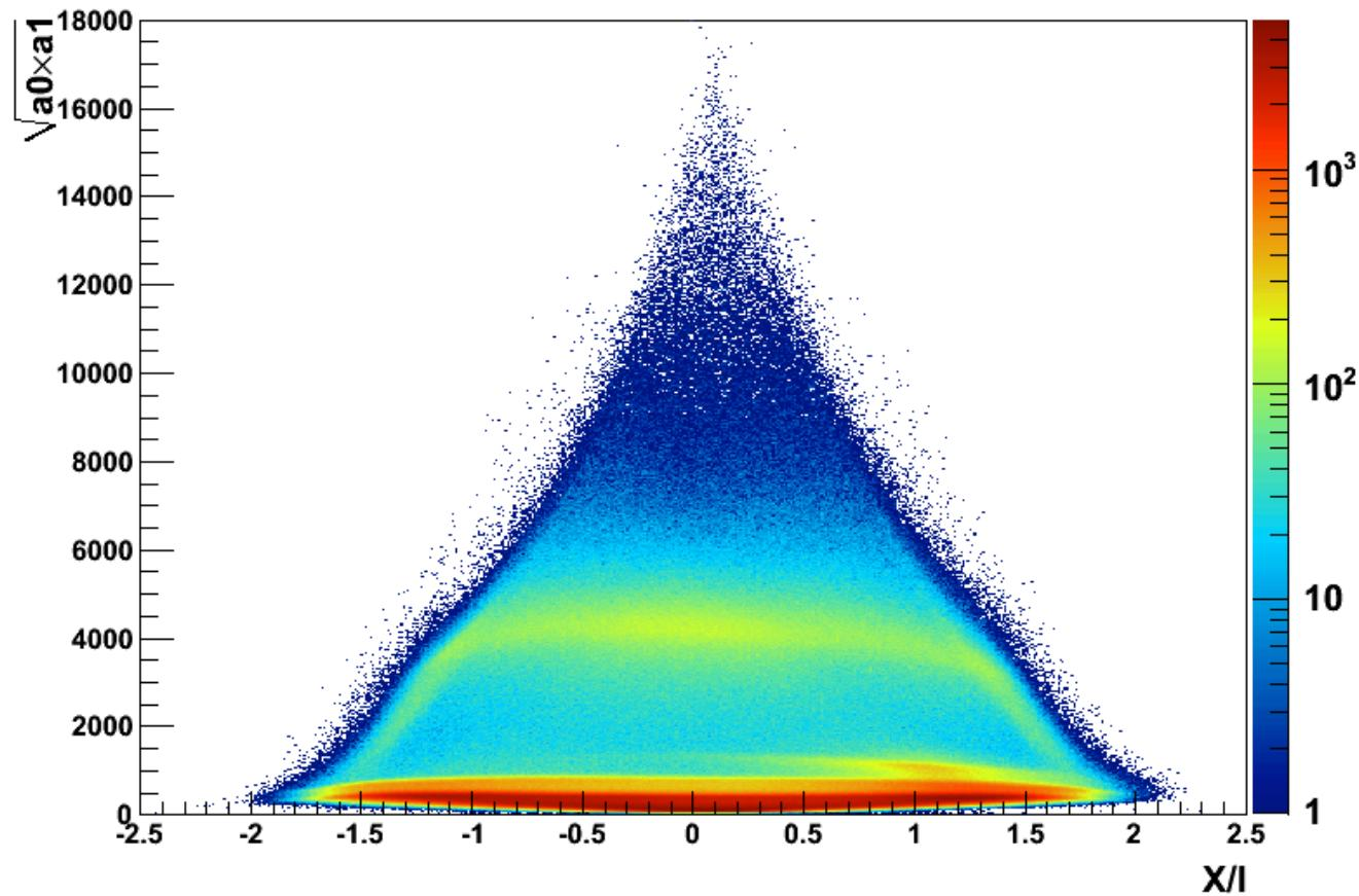
Three calibration source energy: Na22(1.27MeV), AmBe (4.4MeV) and muon minimum ionization peak(~20MeV)
