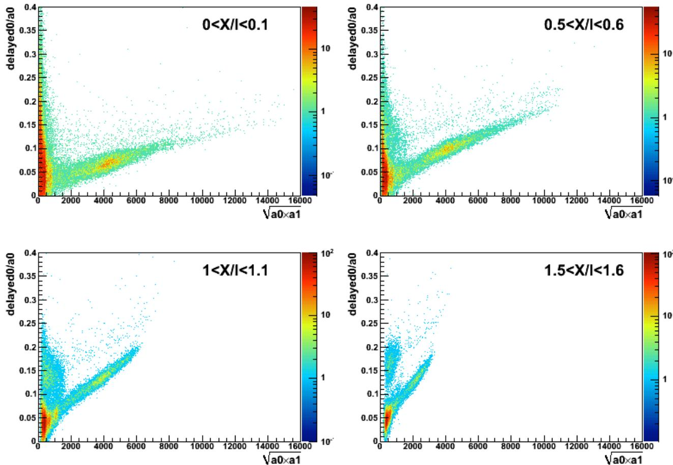
n/g can only be separated in narrow slices along the tube. The n/g separation is getting better when the position is closer to ends.
