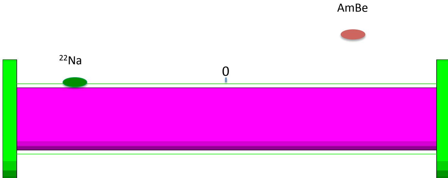
$^{22}\text{Na}$ :  $1.0\mu\text{Ci}$ . Placed at each 2.5 cm along with the tube.
