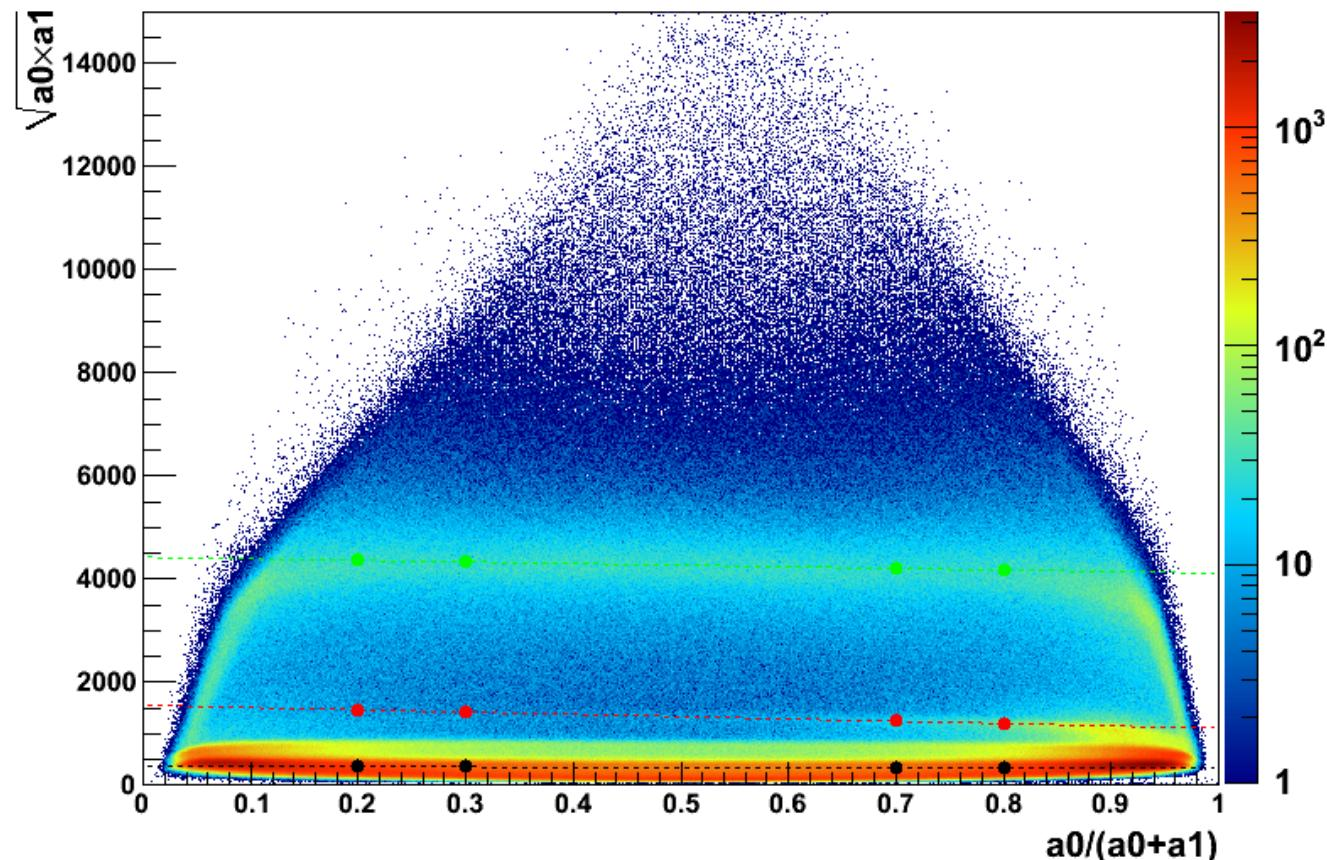
Three calibration source energy: Na22(1.27MeV), AmBe (4.4MeV) and muon minimum ionization peak(~20MeV)
