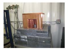
Samples are placed inside shielding next to the sensitive Germanium detector
