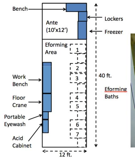
Seven electroforming baths to be installed
