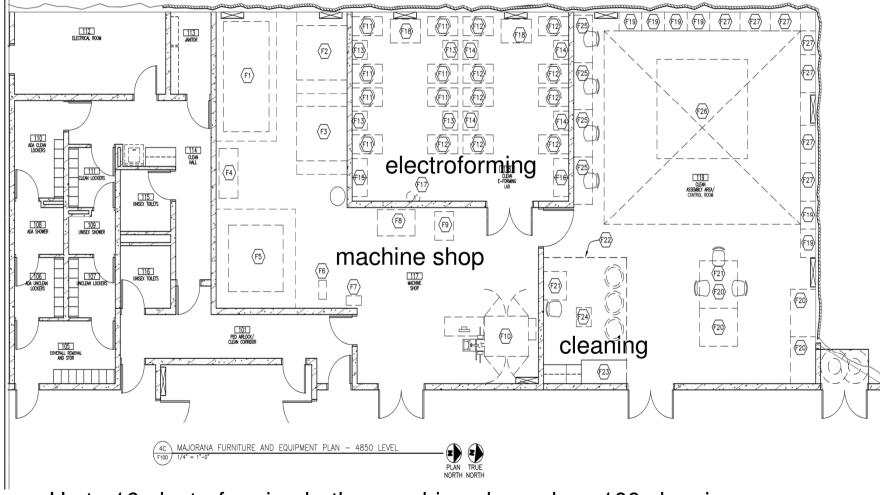
Up to 16 electroforming baths, machine shop, class 100 cleaning area
