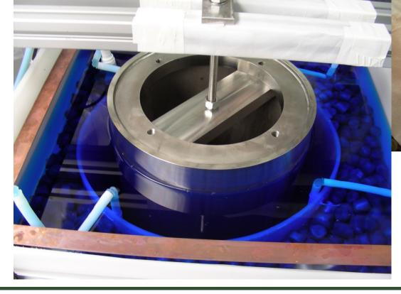
Each bath can produce ~100kg/yr on mandrel shown above (13" diameter x 23" height)
