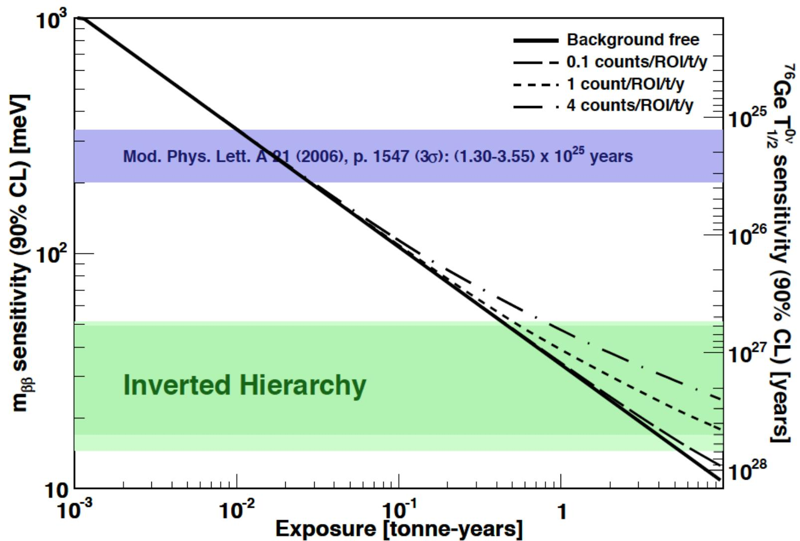
Depth Requirements for a Tonne-Scale  $^{76}\text{Ge}$  Neutrinoless Double-Beta decay Experiment
