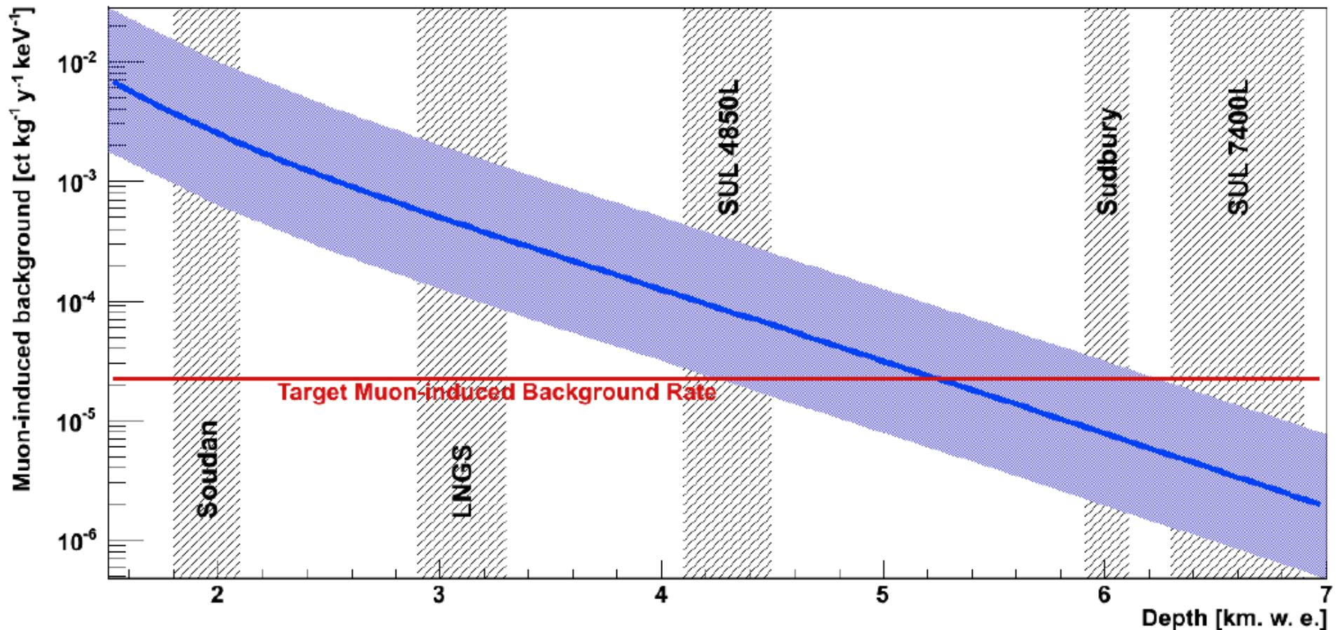
Depth Requirements for a Tonne-Scale 76Ge Neutrinoless Double-Beta decay Experiment
