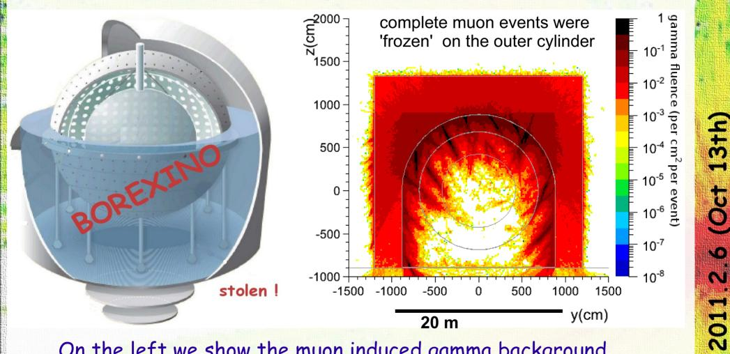
On the left we show the muon induced gamma background present in BOREXINO as predicted by FLUKA note the individual showers visibly penetrating the shielding
