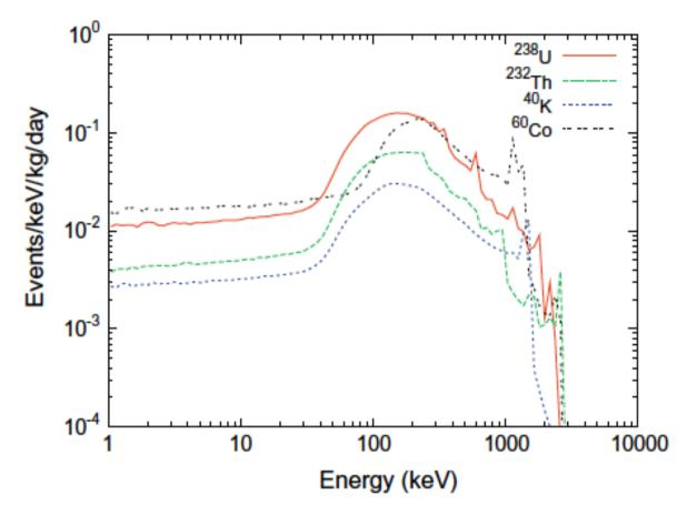
Typical contaminations in low background PMTs: 30 ppb U/Th, 60 ppm K. 10 mBq/kg of <sup>60</sup>Co in copper.
