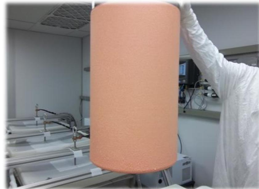
*Inspection of copper being electroformed at the TCR in SURF (above) and the shallow underground laboratory at PNNL (left)*
