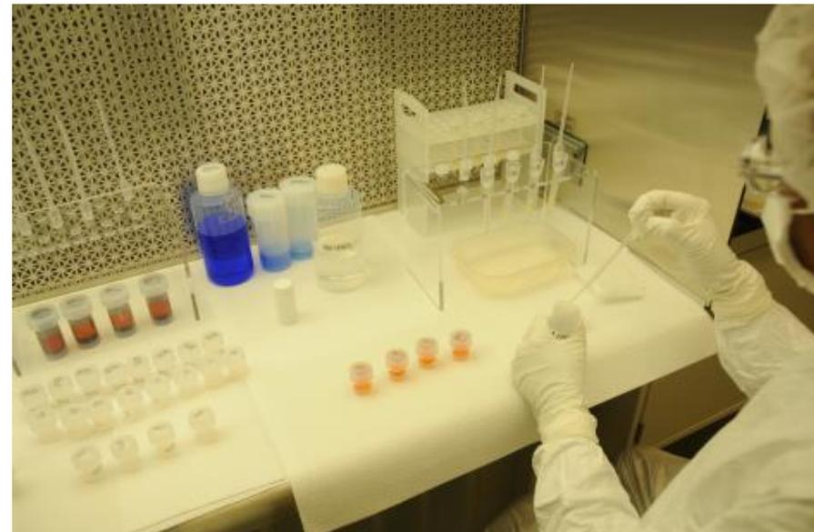
*Preparation of copper samples using ion exchange methods in a laminar flow hood inside a class 10000 clean room*
