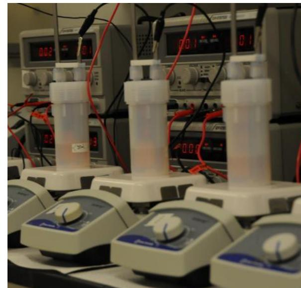
*Preparation of copper samples using the electrochemical method (above) and electrochemical electrodes (below)*
