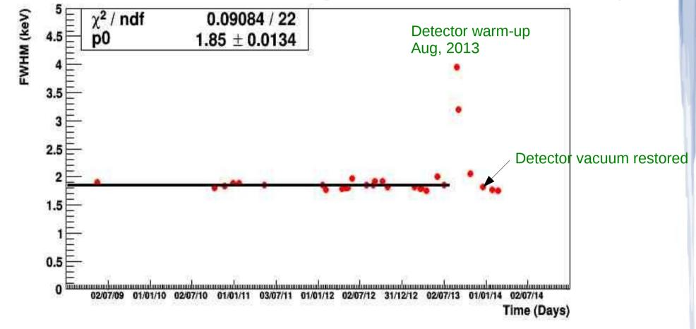
The detector resolution doubled after warming up, all peaks had this feature, after re-establishing the vacuum, the resolution the displayed peak was 1.76 keV FWHM, the long-term average was 1.85 keV FWHM.
