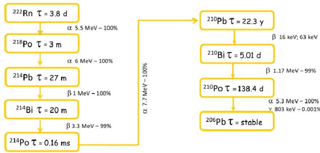
**FIGURE 1.** Radon decay chain
