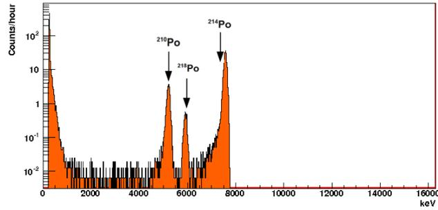
**FIGURE 2.** Energy spectrum of a copper sample exposed to  $^{222}\text{Rn}$  for 63 d.
