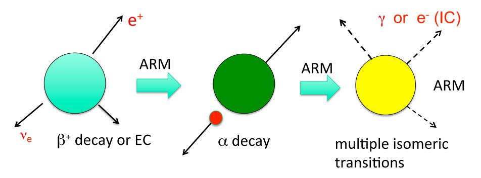
States with  $\gamma$  decay lifetimes < 1 ns would decay immediately in the same step all the way to the ground state
