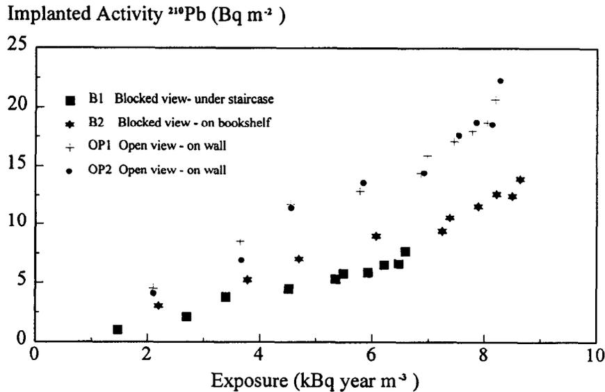
Fig. 1. The growth of implanted  $^{210}\text{Pb}$  in four different framed glass sheets exposed in a radon dwelling for 3.5 y. Each point corresponds to a measurement of implanted  $^{210}\text{Po}$  in the laboratory and an evaluation and exchange of the radon track-etch detectors exposed at the position of each glass sheet.
