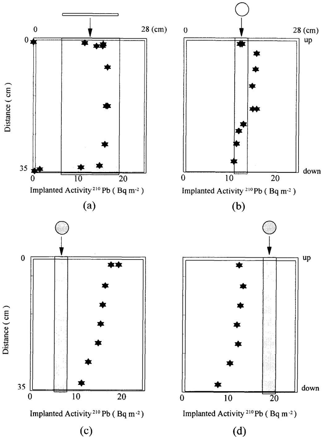
Fig. 3. Results from an activity scan of sample OP2 (a) and B2 (b-d) of Fig. 1. The slit collimator (a) is of the same area as the circular one (b-d) and the scan position is indicated by the shadowed area.
