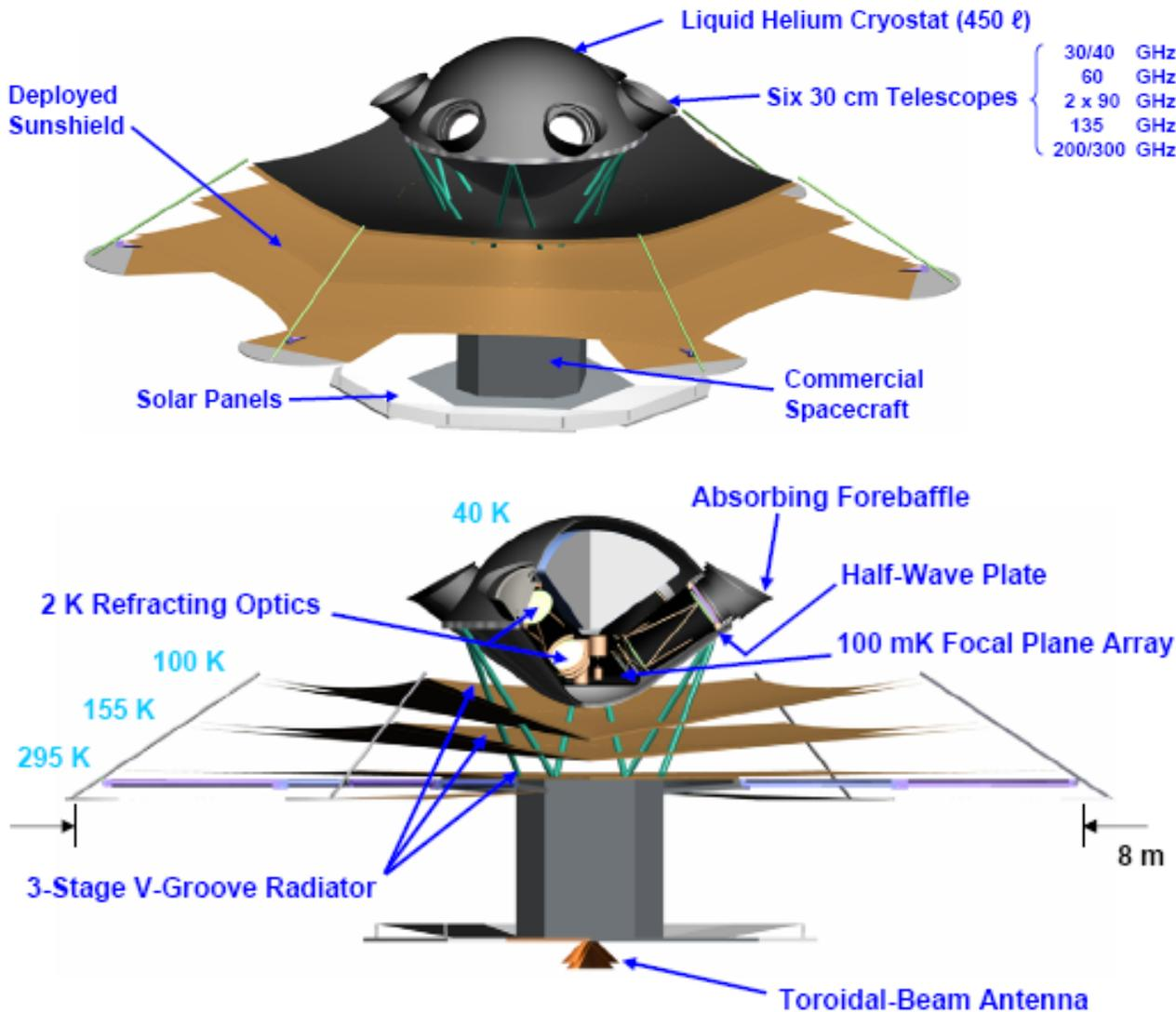
Fig. 2. The EPIC instrument consists of 6 imaging polarimeters. The detailed design for one of the polarimeters is shown in Fig. 5. The telescopes are cooled to 2 K inside a liquid helium cryostat. Bolometric detectors at the focal plane are maintained at a temperature of 100 mK. The cryostat and radiators are mounted to a commercial spacecraft bus through bipods.
