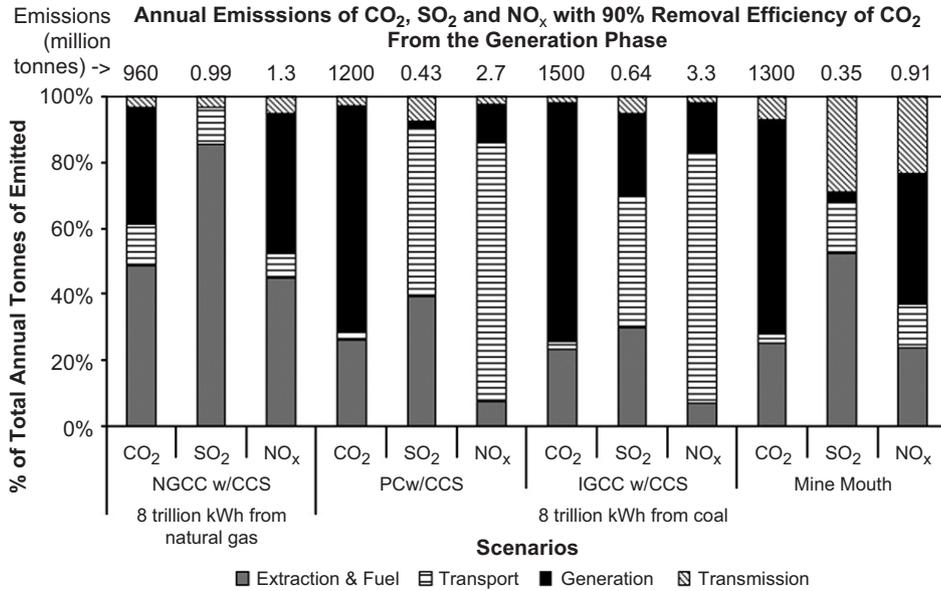
Fig. 5. Emissions of CO<sub>2</sub>, SO<sub>2</sub>, and NO<sub>x</sub> by life cycle stage (assuming 90% removal of CO<sub>2</sub> from generation).
