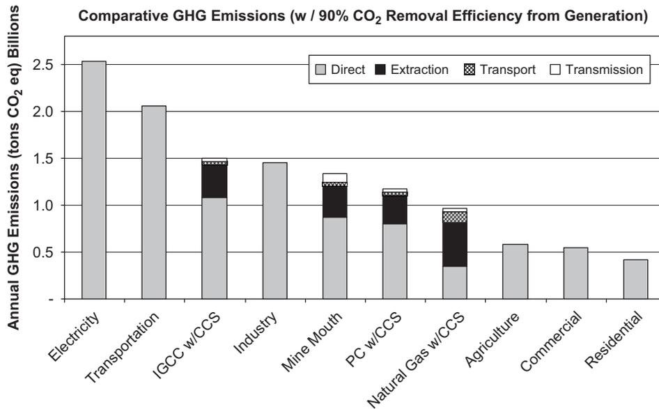
Fig. 6. Comparison of GHG emissions between current economic sectors and future scenarios for electricity production (90% CO<sub>2</sub> removal efficiency in the generation phase of future scenarios).
