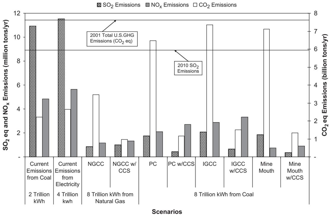
Fig. 3. Annual life cycle emissions (SO<sub>2</sub>, CO<sub>2</sub>, and NO<sub>x</sub>) for coal and natural gas scenarios.
