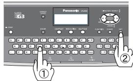
Enter the User portion of the email address and press **SET**. The machine will complete the email address with the Default Domain preprogrammed in the User (Internet) Parameters. (i.e. will add "panasonic.com" to the email address)
