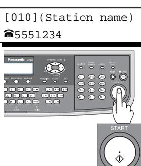
**8** You can now set other Program Keys by repeating the procedures from Step 4, or return to standby mode by pressing **STOP**.
