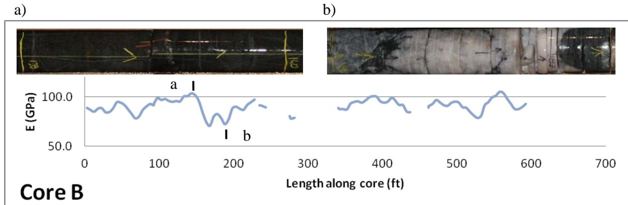
Fig. 6 Plot of E along the length of Core B for only the amphibolites showing the effect of changes in lithology. The gaps reflect the occurrence of rhyolites which are omitted from this plot. a) One foot (.3 m) core of amphibolite which represents the bulk of the rock mass shows a high value of E. b) Example of changes in lithology along the core length which may represent volumes of healed fractures.
