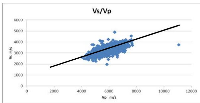
Fig. 3 Plot of  $V_p$  vs.  $V_s$  for all of the amphibolites measured in this study. The correlation between  $V_s$  and  $V_p$  is weak ( $R^2 = .6$ ) but yields a relationship of  $V_s = .4 V_p + 1060$  m/s.
