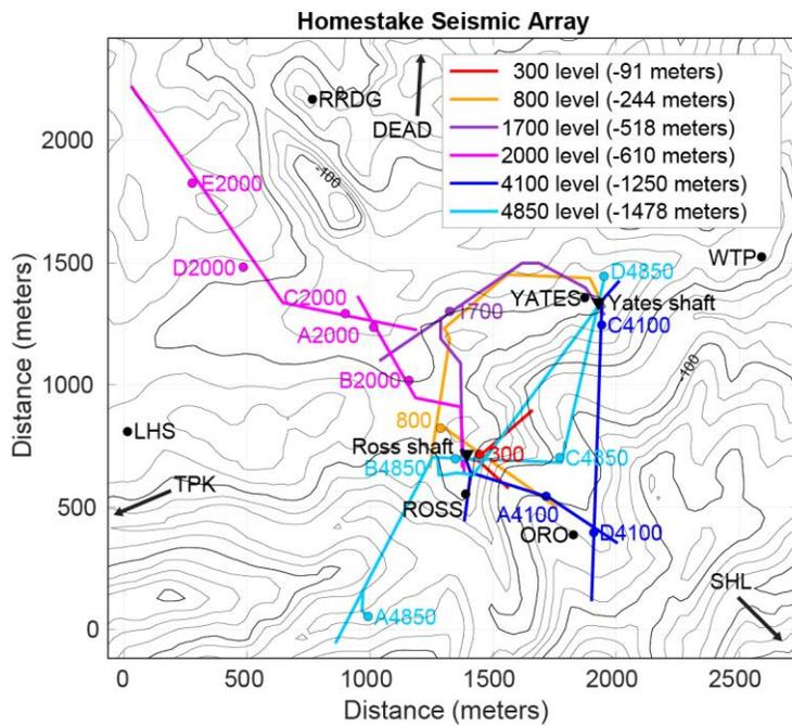
**Figure 1:** Homestake seismometer array layout. The lines of different colors depict the relevant drifts at various depths, along which we installed underground seismic stations. The black filled circles denote the surface stations (remote surface stations DEAD, SHL, and TPK were located approximately 2-3 km outside the depicted region). Also shown are the two shafts at the Homestake mine, known as the Yates and Ross shafts, denoted by black filled triangles.
