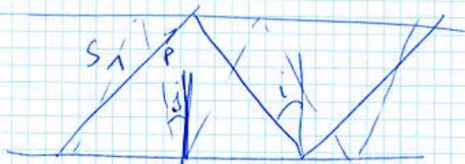
$$\frac{\sin i}{v_s} = \frac{\sin j}{v_p} \Rightarrow \text{different speeds for 2 different waves, but they propagate through the medium in different ways.}$$
