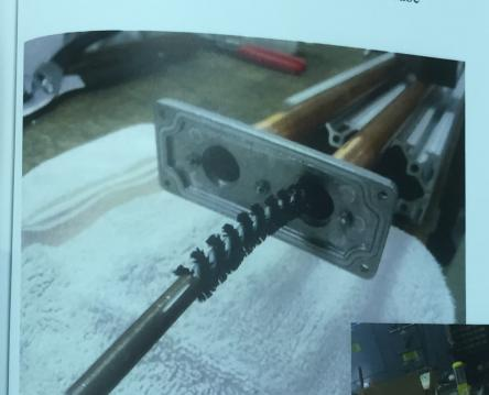
Before Straw Tube Co2 Detector can be assembled, inside of copper tubing must be cleaned out of debris from tube storage, assembly contamination, etccc.
