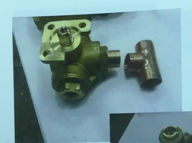
Valve will need to be taken apart to properly clean bronze chips from the milling process. Ultrasonic cleaner is used during this step.
