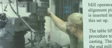
Mill operator then changes alignment pin to end mill. A stop is inserted in mills vice to speed up this set up.
