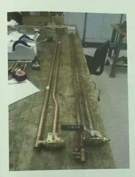
A crude prototype copper tube leak detector was constructed in 2013 and tested
