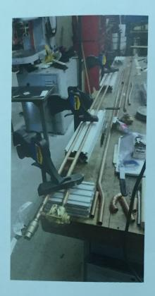
Once Ball Valve end of assembly is sized correctly Solder Paste is added to fittings. A clamp is then placed over the length of copper tubing and held securely.
