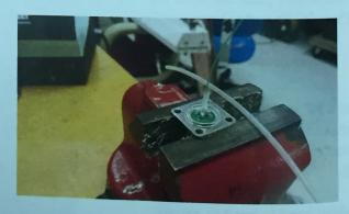
SAWLEC F-POST 4-PINI ARE USED TO CONNECT to COZ DETECTOR BOARD, WIRES ARE COVERED W/ HEAT SHRINK TUBING.
