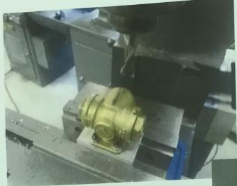
After bronze ball valve is mounted to aluminum fixture the valve is positioned to mill a flat across the casting at three points.
