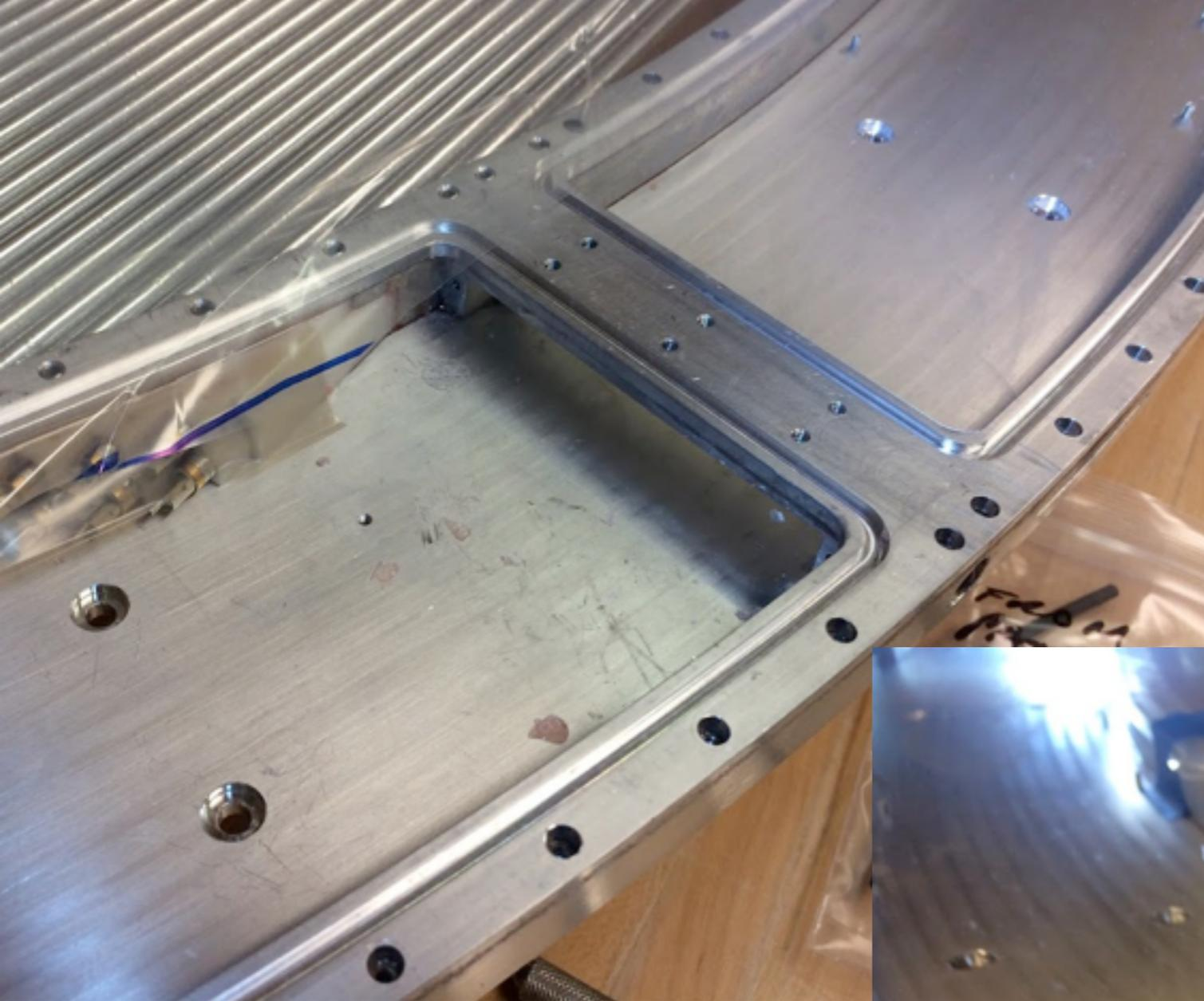
Aug 31-Sept 10: Removing excess epoxy from middle rib to install side panels.
