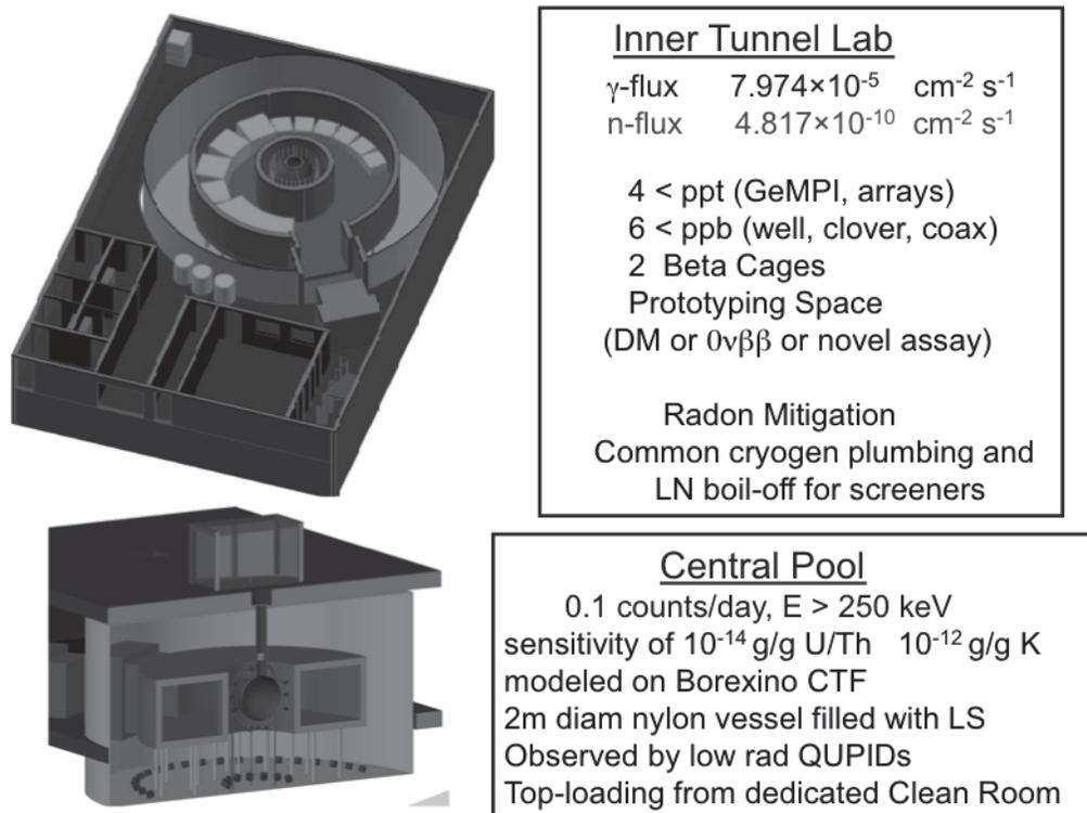
**FIGURE 3.** Cutaway view of the inside of the water shield, showing the location of the screeners in the toroidal inner tunnel lab and the top-loading immersion tank at the center.
