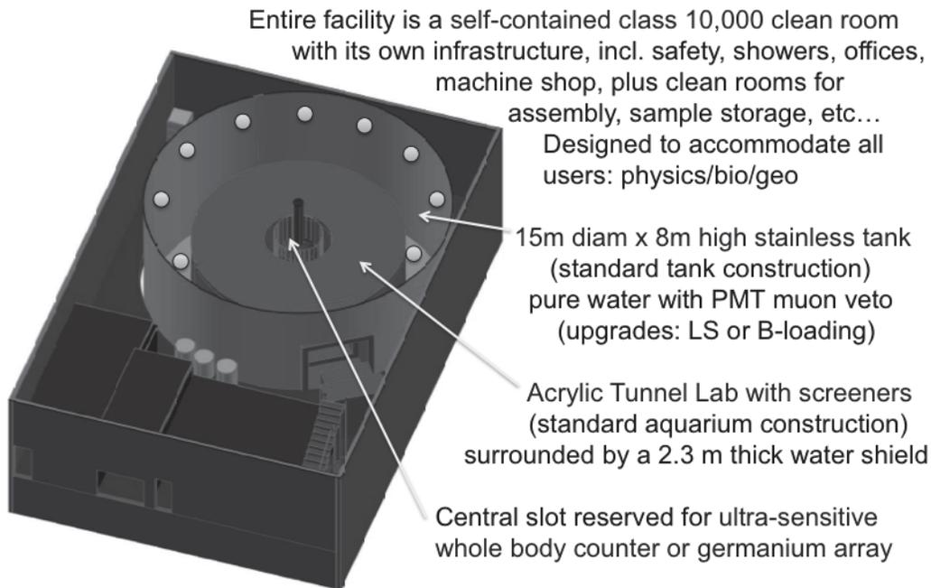
**FIGURE 2.** Rendering of FAARM, showing the water shield and inner tunnel lab.
