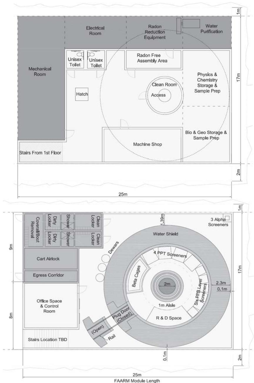
**FIGURE 1.** Floor plan for the DUSEL 4850' level Facility for Assay and Acquisition of Radiopure Materials, or FAARM.
