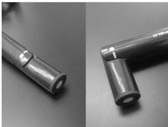
The measurement probes have swiveling tips to allow for more convenient data collection. Note: **that these tips are only meant to swivel in one direction. They will break if they are bent in the other direction, and they are very fragile, so it does not take much to do this.** Please be very careful as these are costly to replace.
