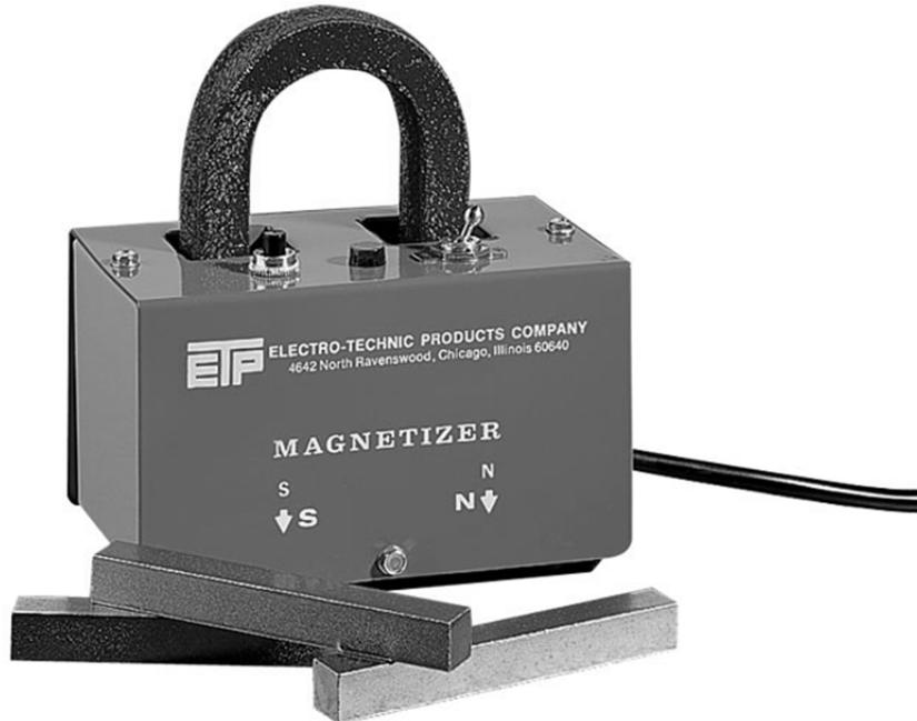
*Important to know is that the magnetizer is poorly labeled.* The N and S do not indicate the end of the magnet that goes into the magnetizer! We believe the company is trying to imply that magnets inserted into the side labeled N will be north attracting and vice versa. You need to insert the S pole of the bar magnet into the side labeled N and the N pole of the bar magnet into the side labeled S.
