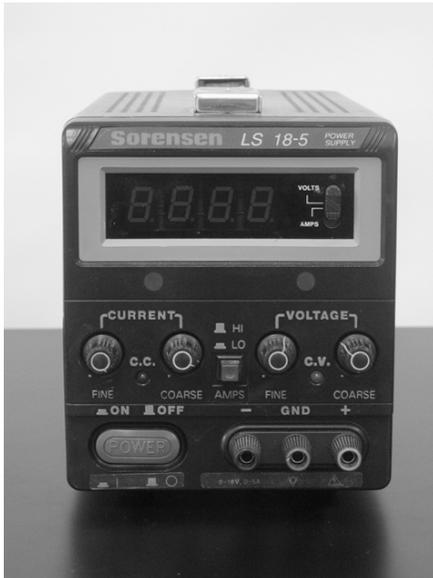
The 18volt 5 amp power supply is an all-purpose power supply for the production of constant currents and voltages.
