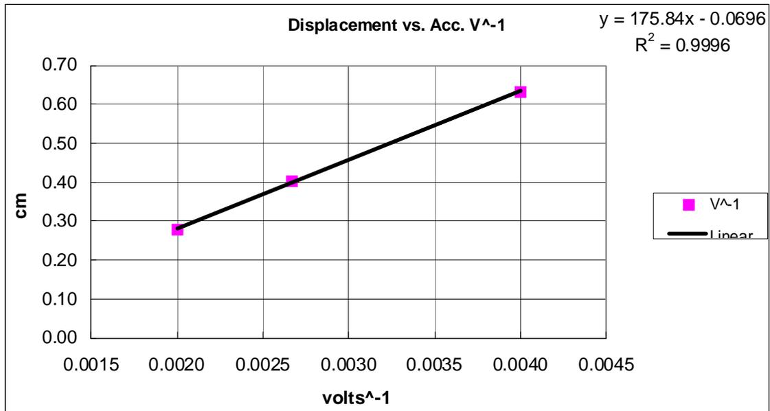
This is a linearized plot of the displacement as a function of accelerating potential
