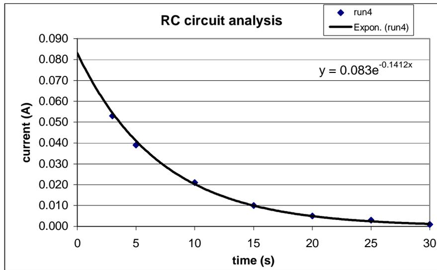
The time constant  $1/RC$  for the circuit was calculated using  $R(\text{effective})$ .  $R(\text{effective})$  was found using the initial current extrapolated from the graph.
