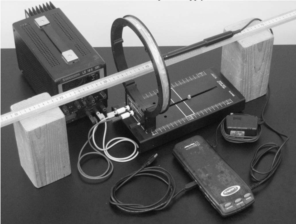
*Problem 6* – Pasco large coils and base, wood blocks, banana cables, Hall probe, SensorDAQ interface, meter stick, 18V/5A power supply
