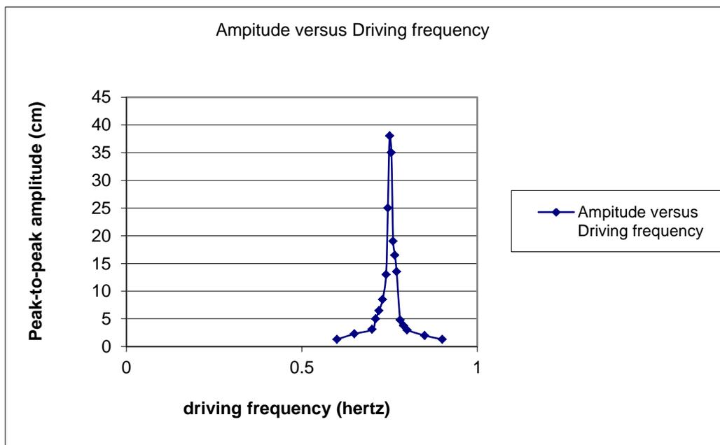
The peak here is at 0.75 Hz, with measured amplitude of 38cm.
