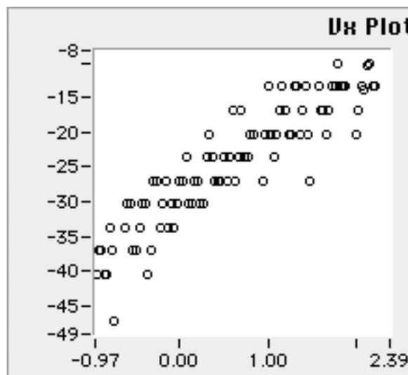
Again we include an “autoscaled” graph (on the right) and one we scaled by hand. There is obviously a non-zero slope in these velocity-versus-time graphs, along with the scatter discussed previously. After seeing this plot, it is more apparent that the velocity-versus-time graph for the good movie is that of constant velocity.
