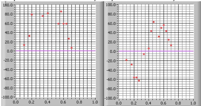
The data from the video measurements were assembled into the following graph. The pendulum becomes less ideal for greater release heights.
