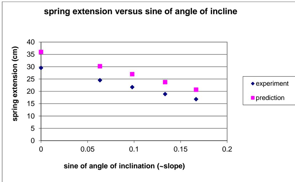
The trend in the prediction and the measurements look the same. The consistent slight difference or shift in the data points might be due to friction.
