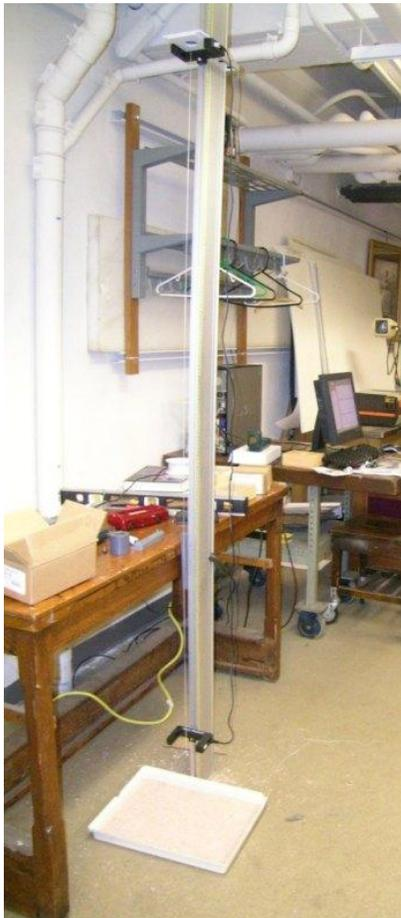
The photogates have two modes: using internal and external light sources. Only use the internal source. You can switch to this mode by unblocking the detector on the inside of the photogate.
