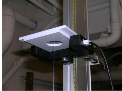
A plumb-bob and cylinder were made to fit into the platform. The plumb-bob will be used to align the photogates in the setup. The diameter of the cylinder is just over 1". When aligned correctly, this will produce drops that do not miss the gates and are repeatable to about 1 millisecond if your gates are over 1 meter apart.
