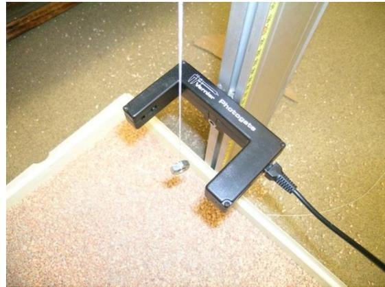
The major challenge here is properly setting up and aligning the gates. **Note that this must all be done very carefully to observe the effects of air resistance. For example, for a fixed drag coefficient (using balls of identical diameter), a solid plastic ball will take about 3 milliseconds more to fall 1.5 meters than a steel ball. This type of precision can be achieved with care. This is an excellent lab.** Lean on the students to do it well and they will learn a lot.
