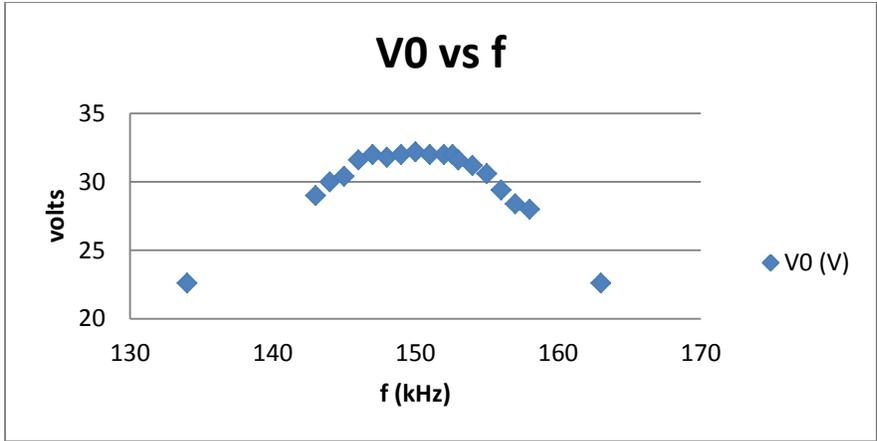
Figure 41: Step 1, part D a much broader resonance peak due to the large resistor added. Measured Q (5.26) implies a series resistance of 1850 ohms, compared to the measured 2050 ohms over the resistor and inductor.
