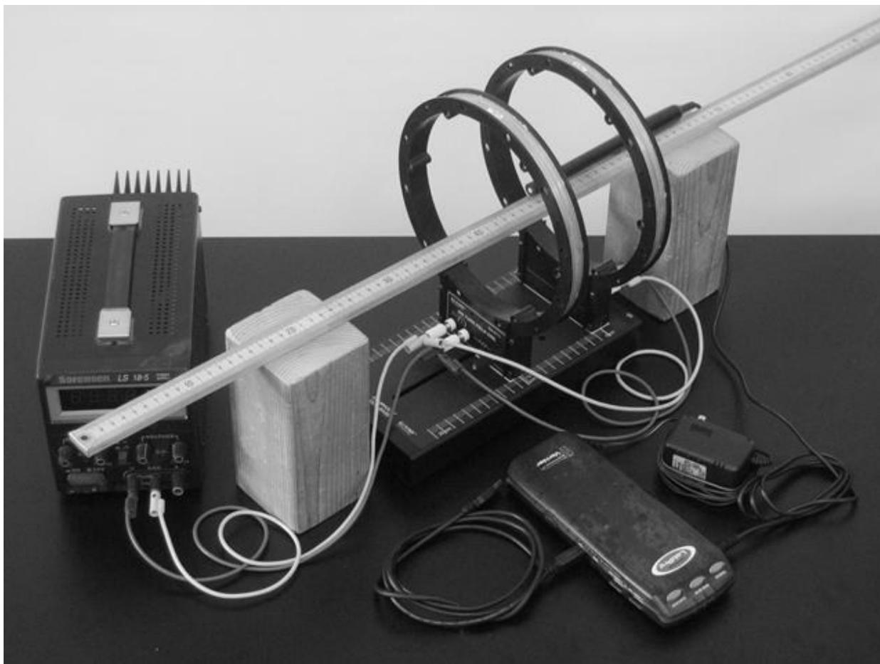
Figure 19: set-up for the Helmholtz coils.
