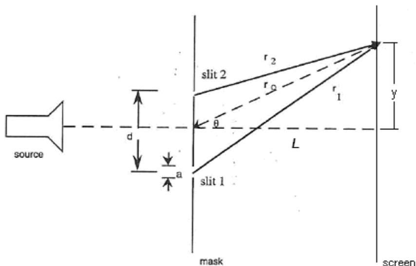
Because of the dimensions of the apparatus and the wavelength of light, we can make some very simple approximations. Refer to the diagram above. Very close the slits, the two emerging beams are almost parallel. For some position,  $y$ , along the screen, the path difference,  $\delta$ , between the two beams is
