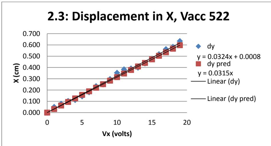
Figure 11: Displacement vs voltage over x-deflection plate for measured (dy) and predicted (dy pred) values. Made with L=2.0 cm and D=4.75.
