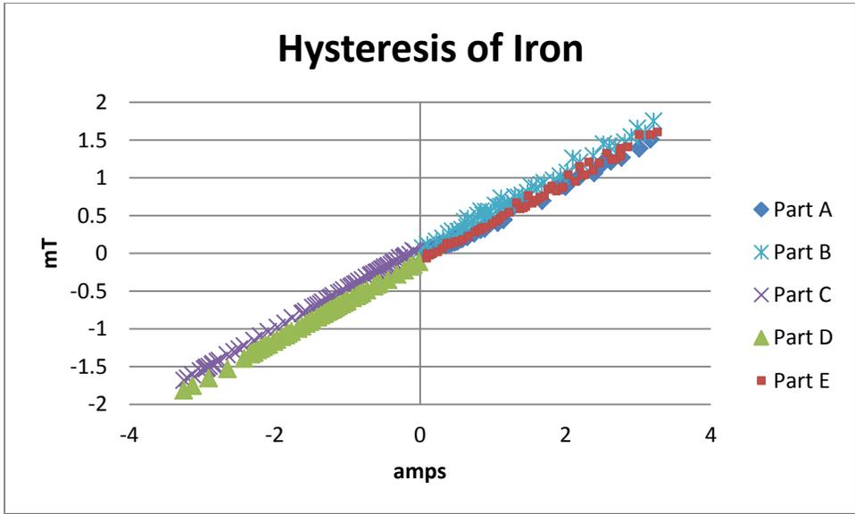
Figure 29: Hysteresis curve for soft Iron. Soft iron has almost no hysteresis, it will immediately align with the field.
