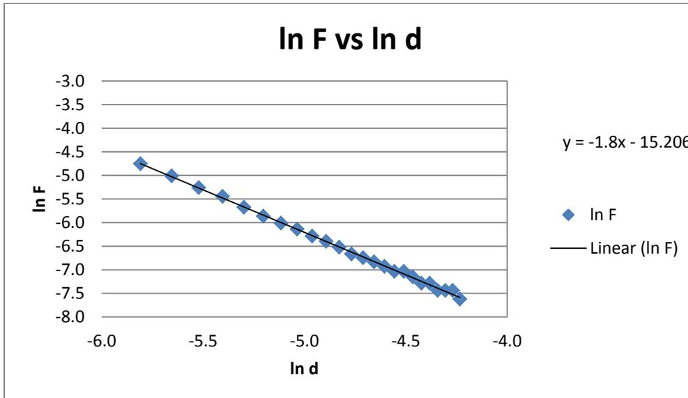
Figure 14: log-log plot of Force vs distance. Implies that distance is raised to the -1.8 power and that  $\epsilon_0 A \frac{V^n}{2} = e^{-15.21} = 2.490 \times 10^{-7} \text{ [N}\cdot\text{m}^2]$ . Data was plotted only after  $d=3 \text{ mm}$ , as the data before this was unstable. Voltage was kept at 1040 volts.
