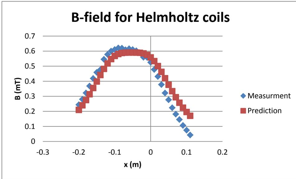
Figure 22: Helmholtz data for measurement and prediction. Here  $x=0$  is for the center of one of the coils. Its possible that background magnetic fields are still responsible for the disagreement.
