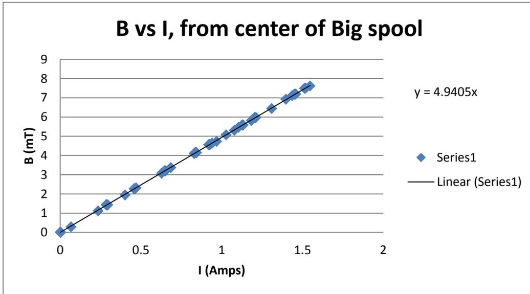
Figure 26: B vs I, can be used to calculate the number of loops ( $N \approx 600$ )
