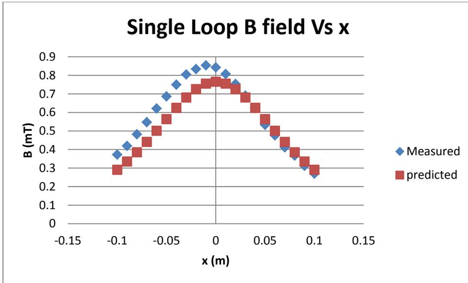
Figure 20: Data and prediction for the single loop. The deviation from predicted is likely due to background field changing along x.
