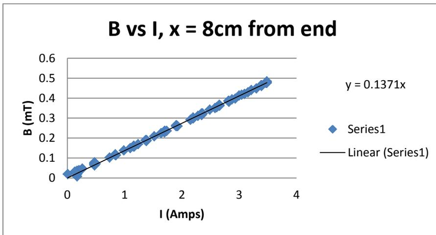
Figure 27: B vs I at a distance of 8 cm from the end.
