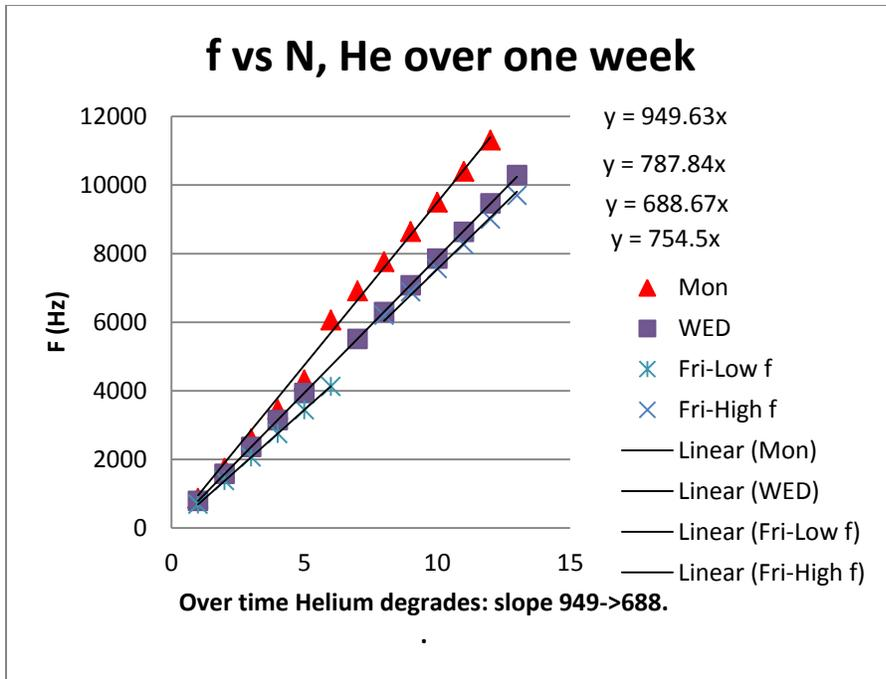
Figure 2: F vs N for Helium over a week of testing. As time goes on, the slope decreases. Also note the 'gap' around node 6. The friday data was split up to investigate this and show that the higher node data was more accurate. Equations on plot are in same order as data series.
