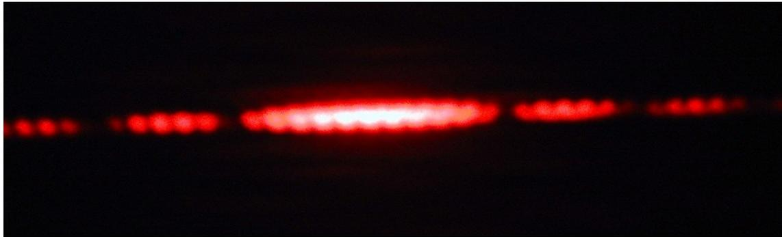
*Figure 1.3.1: A double slit diffraction pattern. The large scale pattern (causing 5 distinct bright patches) is from the single slit diffraction, while the much smaller pattern (making it look like a string of 'bubbles') is from the double slit interference. Students will be able to get a MUCH sharper image than this.*
