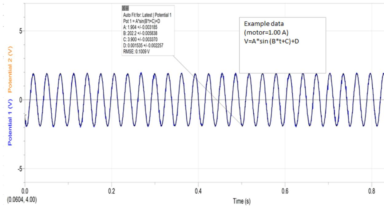
Figure 36: voltage vs time, fit to find amplitude and omega
