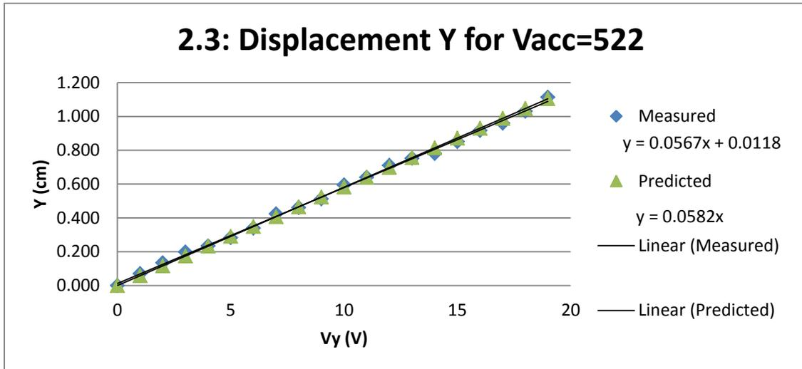
Figure 10: Displacement due to Y-deflection plates.
