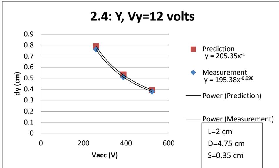
You can also plot vs  $V^{-1}$ , especially if they are having troubles fitting a power equation to it. Students will try and fit a linear line to the  $1/V$  line, and try to pass the bad fit off as bad data. Do not accept this.
