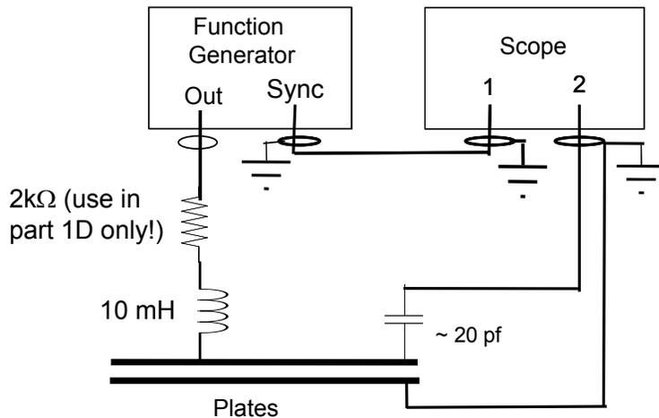
Step 1: Resonance: Students should be able to set-up this circuit with minimal difficulty. It is important to make sure that all the grounds are the same. You can set the oscilloscope to measure Pk-Pk voltage and phase of channel 2 to get these measurements easily. Finding the resonance is as simple as finding the maximum Pk-Pk value.
