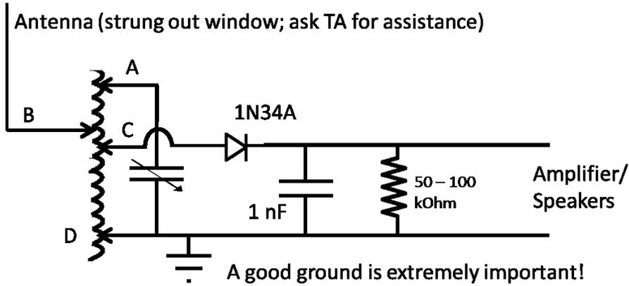
Figure 46: figure 6.6 from manual, the final radio.
