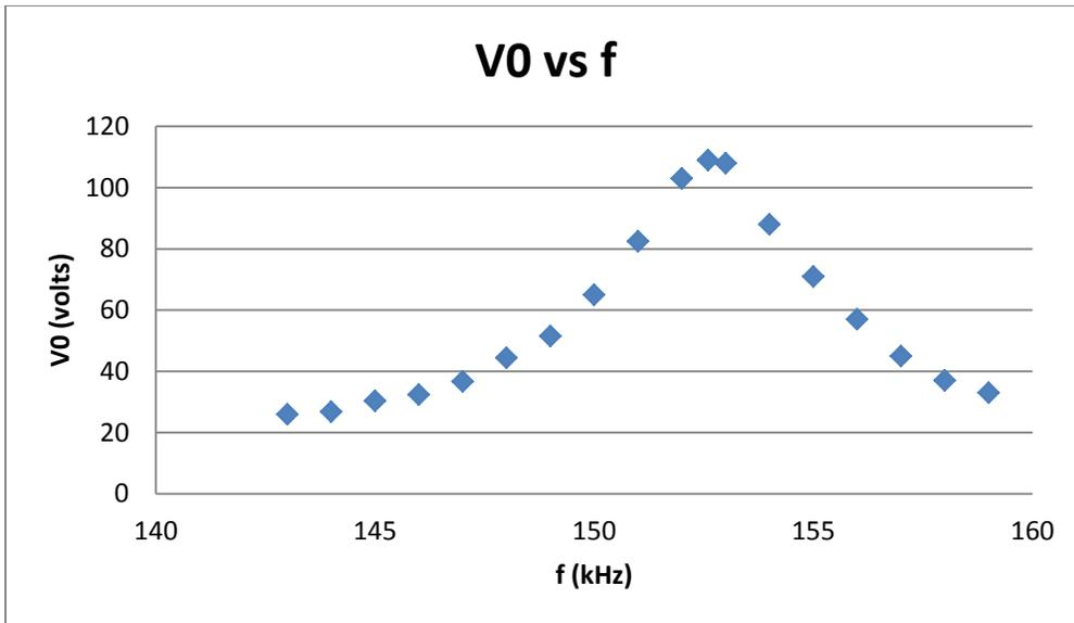
Figure 39: Part 1, step C, resonance plot. Measured  $f_0 = 152$  kHz, predicted was 199 kHz. Measured Q (30.52) implies a series resistance of 320 ohms, only 66.4 ohms are measure over the inductor. The extra resistance is inherent to the function generator.
