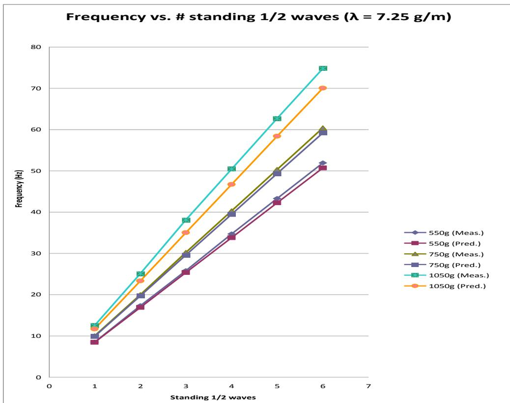
Figure 1.1b: Predicted vs measured  $f$  Vs  $N$
