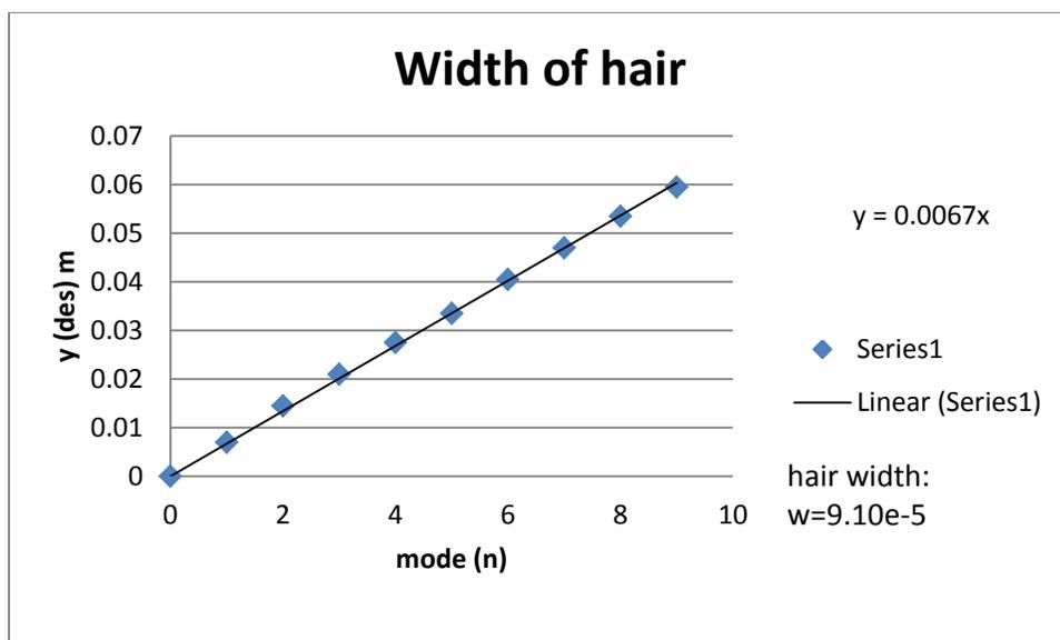
**Step 3**, Double slit: It is difficult to mark and measure the individual distances for each node, but it is fairly easy to count how many nodes are in a given distance. If they can measure the total length of 20-40 nodes, they should get pretty good results using the  $\Delta y_{ave}$  calculation. Single slit diffraction can cause dark points where seeing dots is difficult. If they can still make them out, encourage students not to stop at these points. More data is more important.
