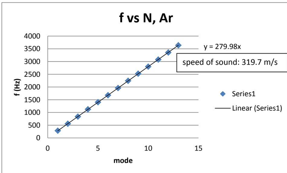
Figure 1: Plots of f vs N for Nitrogen and Argon. Note: The slopes are deceptively similar to the speed of sound, but NOT exactly.
