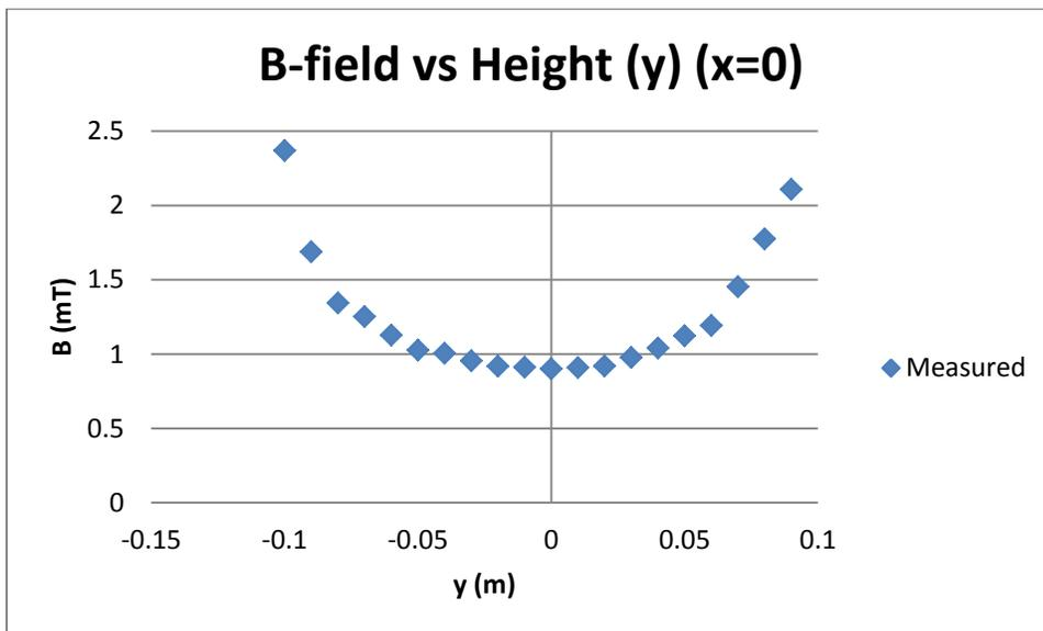
Figure 21: Vertical data for the single loop. This is what students should qualitatively predict. The data here ends at the loop itself.
