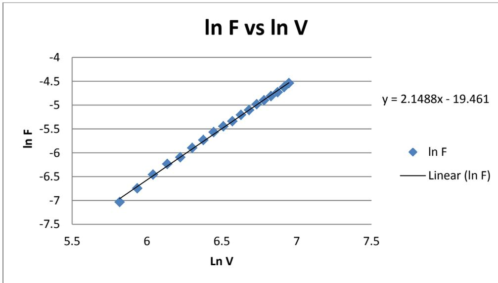
Figure 15: Log-Log plot of force vs distance. This implies that Voltage is raised to the power 2.15, which is within uncertainties of 2. Intercept implies that  $\epsilon_0 A \frac{1}{2d^m} = e^{-19.461} = 3.533 \times 10^{-9} \text{ [N/V}^2\text{]}$
