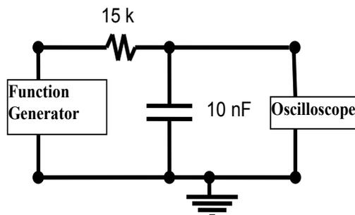
Figure 3.3.1: Integrator circuit
