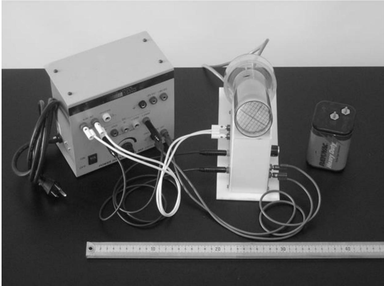
Figure 9: the set-up of the CRT. Note that this diagram uses the variable plugs in the lower right of the power supply for the deflection plates. Do not do this as the standard power supplies are much better for the deflection plates.
