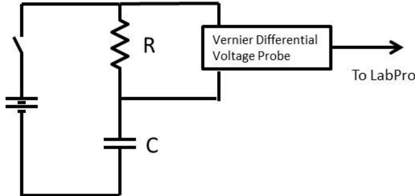
Figure: 3.1.1 Basic set-up for Problem 1. You will be changing the values of R and C as well as the location of the voltage probes.
