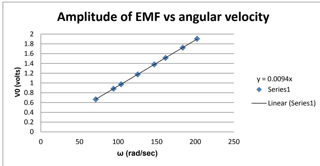
Figure 37: Data from lab 5.2. The slope (0.0094) should be equal to  $NBA$ .  $N$  is given (4000 turns),  $B$  can be measured (0.5992 mT), but measurement of  $A$  is not obvious. This slope implies an area of  $0.00392 \text{ m}^2$ , which falls within the range of the interior area ( $0.0032 \text{ m}^2$ ) and exterior area ( $0.0059 \text{ m}^2$ ) of the loop.
