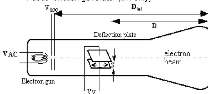
This is a simplified version of the interior of the CRT. It does not show the x-deflection plates, which are in fact in front of the Y-deflection plate.
