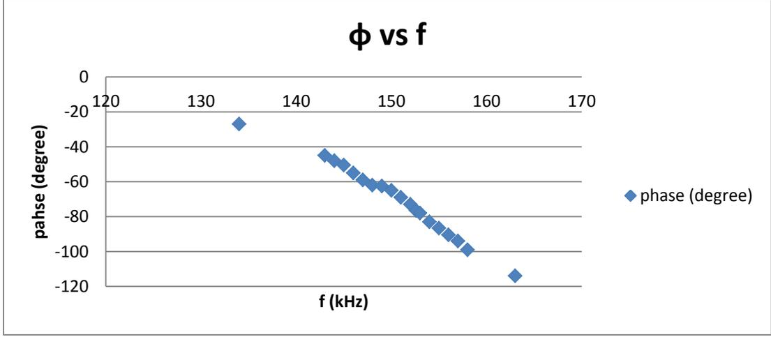
Figure 42: Part D: with the increased resistance, the phase vs f plot is much closer to a straight line.
