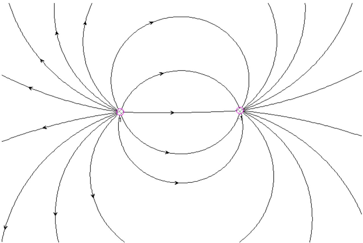
Figure 8: 2-dimmesional di-pole (using vertical line charges). Should be more similar to Lab 2.2 results
