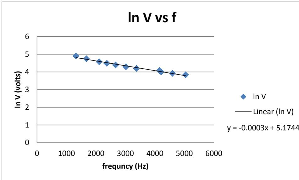
Figure 17: measured RC=0.0003 sec, predicted RC=0.0002 sec.
