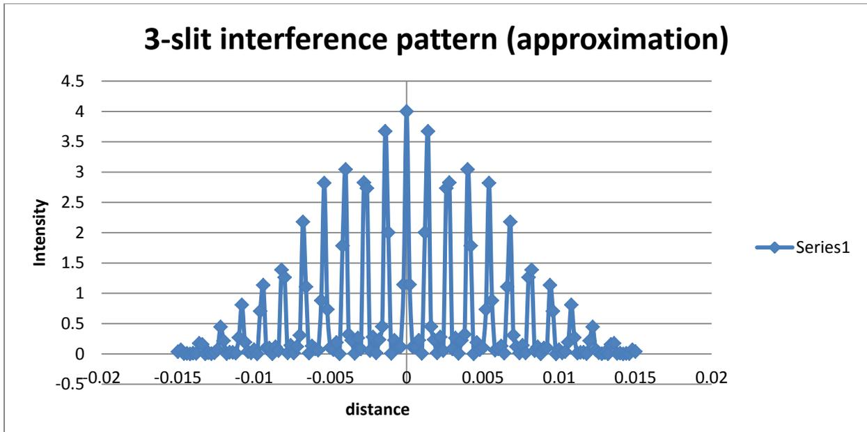
Figure 5: Simulated intensity for 3 slits (only the first diffraction 'envelope').
