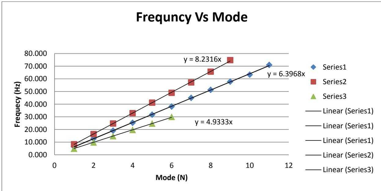
Figure 1.1a: A sampling of  $f$  vs  $N$  for a number of wires and tensions. Series 1: Red wire with 150g, Series 2: Red wire with 250g, Series 3 with 250g
