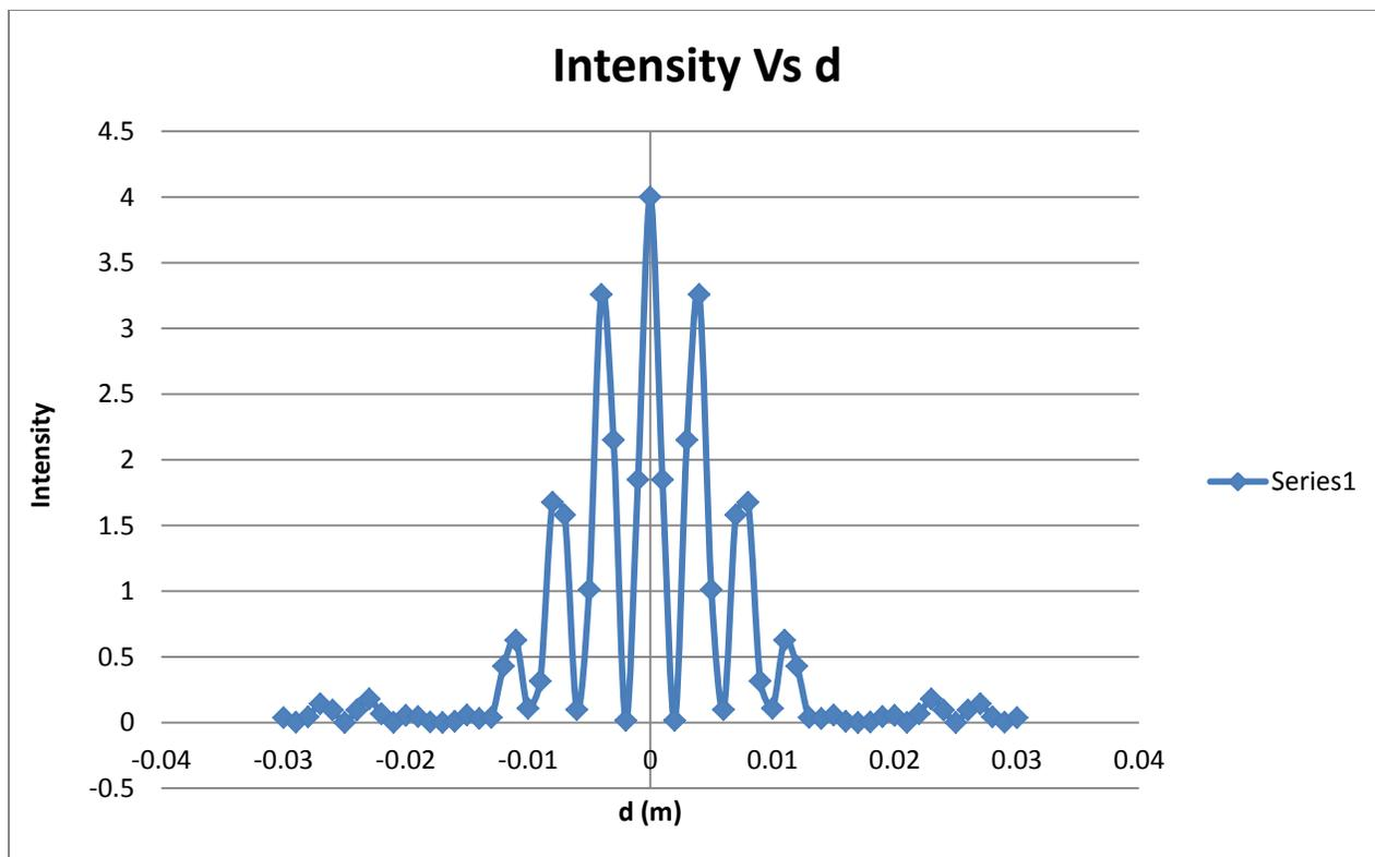
Figure 4: A plot of intensity simulated using the provided equation (step size 0.001 m). It's important to make sure the steps in the points are fine enough that it shows all the detail. Connecting the dots with lines is also important for seeing the desired shapes.
