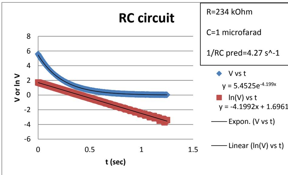
Figure 13: examples of both types on one graph. The measured value of  $1/RC$  is taken from the exponent for the  $V$  vs  $t$  plot, and the slope for the  $\ln V$  vs  $t$  plot.
