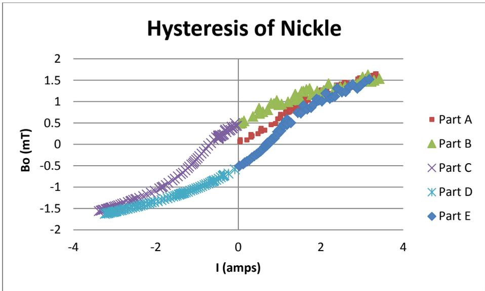
Figure 28: Hysteresis curve for Nickle. Note the wide thickness of the curve implying its high coercivity.
