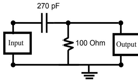
Figure 3.3.2: The differentiator. Note positions of the capacitor and resistor. This is important when using the scope, for which the negative terminal is always ground!
